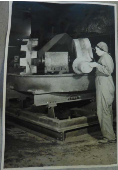
Banding the armature of an Electric Motor in a Banding Lathe.
