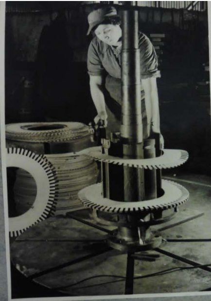
Females are employed on a wide range of opera- tions in the manufacture Electric Motors and Control Gear for Marine machinery, to which they quickly adapt themselves. Photograph shows assem- bly of discs on Armature Hub for a 300 K.W. Elec- tric Generator.
