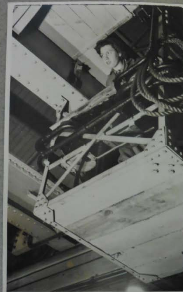
The driver of a 15 ton overhead electric trav- elling crane watching her load. Her crane serves part of the Main Engine Erection Shop and great care and acc- uracy is essential in the operation of this crane.
